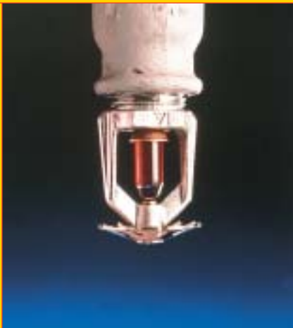
Figure 10 Typical sprinkler head configuration. The red colour of the volatile liquid indicates that the glass will break at 68°C. This is the most common activation temperature.
