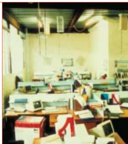
Figures 54, 55, 56 Office fire loading supplemented with wooden cribs produced the most extreme temperatures in any of the six fire tests. Despite this, the unprotected steel beams (which reached temperatures in excess of 1100°C) and floor did not collapse.
